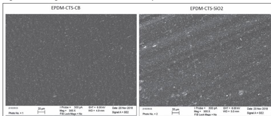
**Fig. 7: STEM/EDX images of CB-filled compound.**
