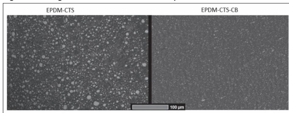
**Fig. 6: SEM image of CB and silica-filled compounds.**
