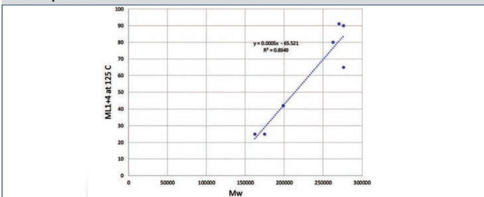
**Fig. 8: Correlation of Mooney viscosity at 0.05 rpm to the Mw. Some investigators have claimed that this should be a very good correlation, but it was not for the EPDMs tested.**
