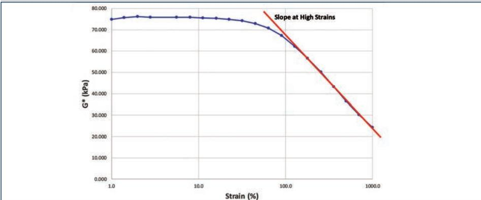
Fig. 23: The slope at high strains for all EPDMs correlates to the Mw value. The value becomes more negative at higher Mw values probably due to more distortion in the sine wave at higher strains which produces a loss of signal in the 1st Harmonic.
