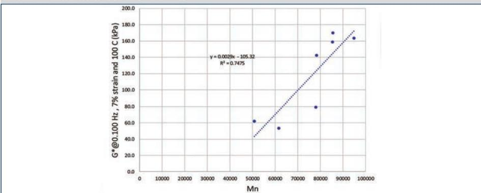
**Fig. 15: Correlation of G\* at 0.1 Hz, 7% strain and 100°C to the Mw. The results show a very good correlation but there are two clusters.**
