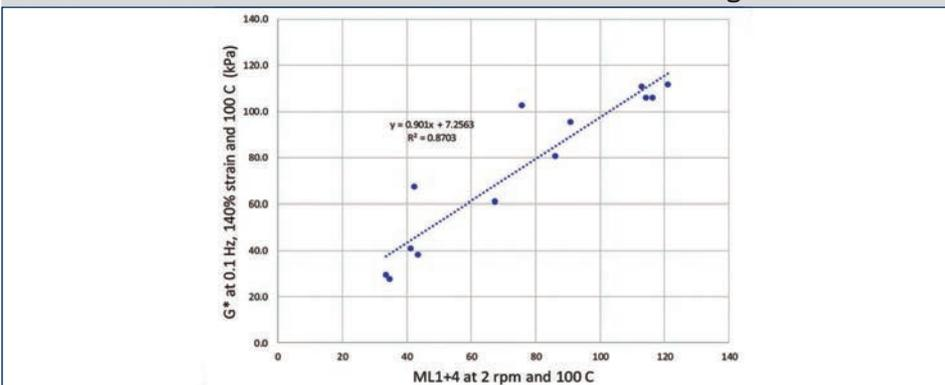
**Fig. 14: Correlation of G\* at 0.1 Hz, 7% strain and 100°C to the Mn. The results show the correct trend with a lot of scatter.**
