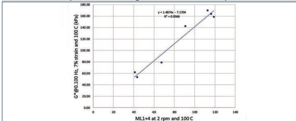
**Fig. 11: Correlation of RPA G\* at 0.1 Hz, 7% strain and 100°C (1st Condition in D6204A) versus ML1+4 at 2 rpm and 100°C. with all 13 EPDMs. Results were very good with the exception of one EPDM.**
