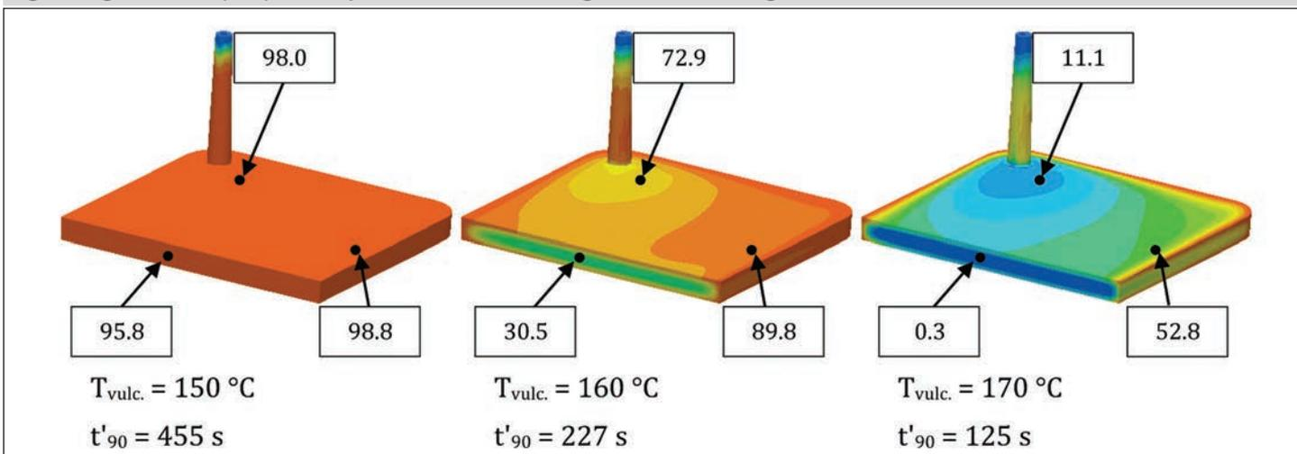
**Fig. 5: Degree of cure (in %) of simulated SBR parts considering a  $\Delta t_{90}$  of 227 s and a deviation of  $\pm 20$  s as batch variation.**
