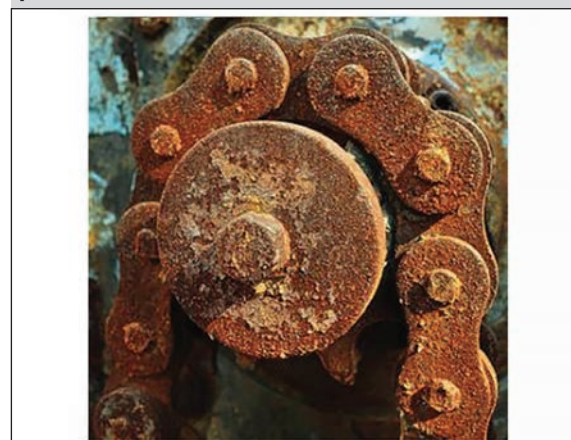
Fig. 5: Rust, grease and oil can cause maintenance problems with standard chains.
