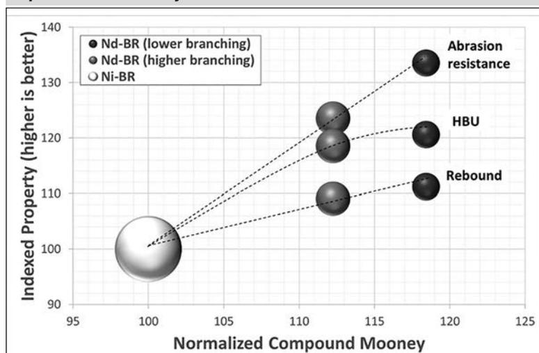
**Table 5:** Performance overview of different high-cis Nd-BR with different molecular architecture. The traditional reference BR has a mainly linear structure.
