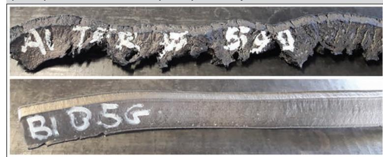
**Fig. 10:** Samples of uncured compounds extruded through the Garvey die of a laboratory extruder. The adopted compound formulation is for tire sidewall. Polymers involved are BR/NR in ratio 50/50; filler type is N375 in amount of 45 phr. Mooney 60 polymers (Neocis BR60 and Neocis BR61EP) are compared with Mooney 40 material (Neocis BR40). The Garvey extrusion test was carried out at 20 rpm and 90°C on uncured compounds.
