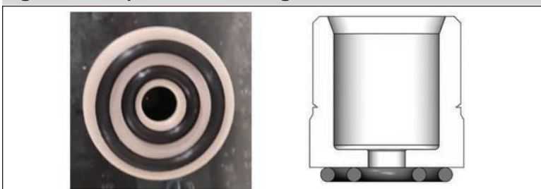
Fig. 8: The set up for the double O-ring test.
