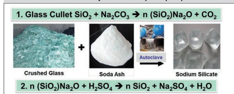
Fig. 2: Silica manufacturing of (1) silicate production via the wet autoclave process starting with cullet (crushed recycled glass), followed by (2) controlled acid neutralization to synthesize amorphous precipitated silica.
