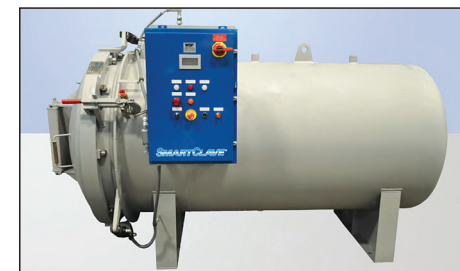
WSF Industries' SmartClave control system mounted on a horizontal autoclave.
