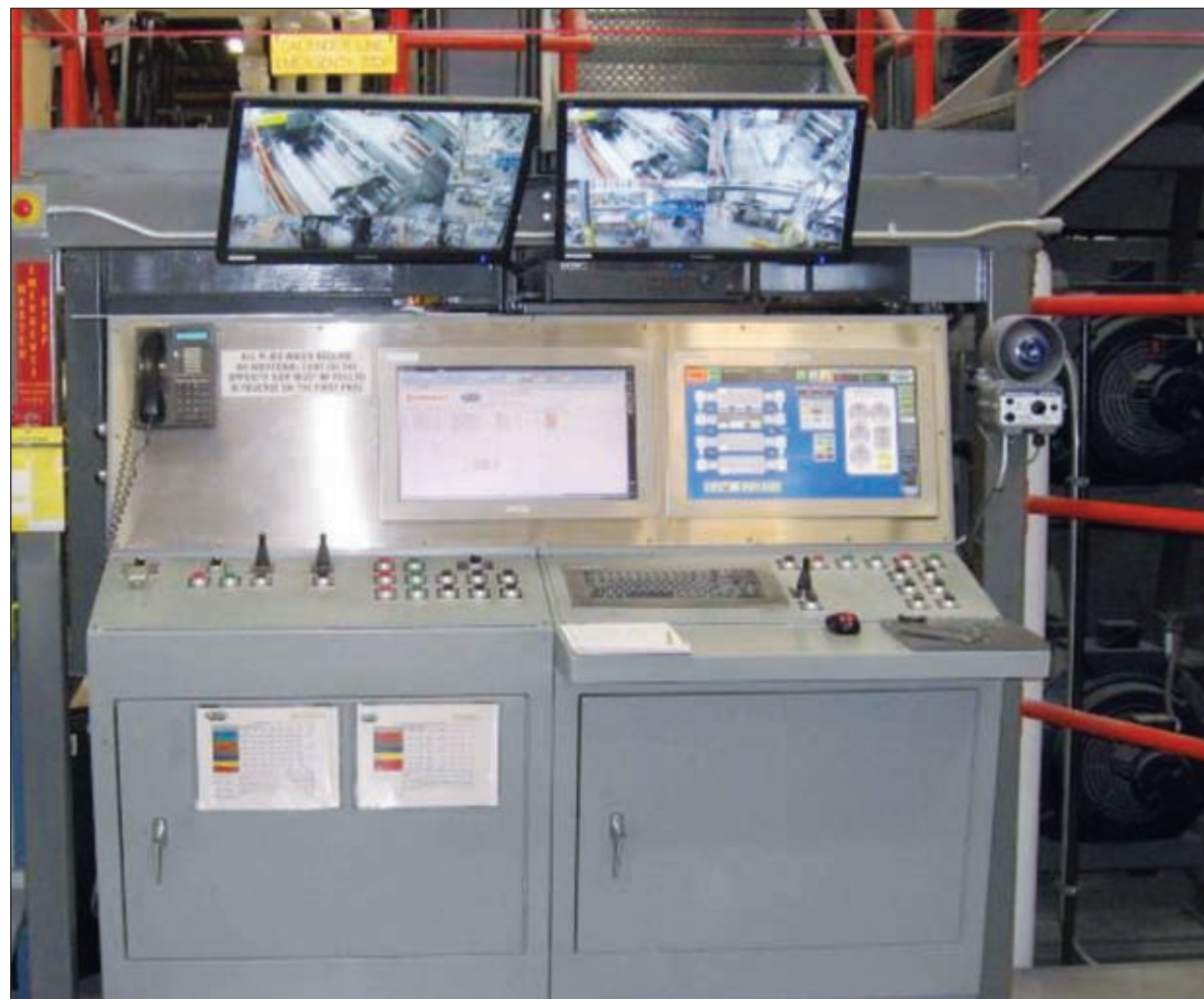
Fig. 16. Contemporary calender line control desk. Digital data display on flat screen VDU, touch screen HMI; Video display screens for monitoring rubber feed to calender.
