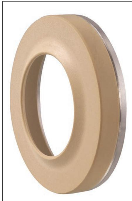
**Fig. 3. The Hygienic U-sit, a metallic flat seal and elastomer seal in one component, provides FDA-compliant sealing screw connections, based on hygienic design.**
