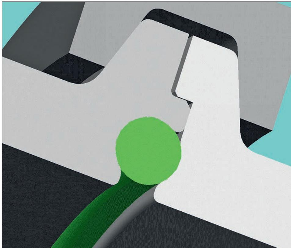
**Fig. 2. Dead-space-free radial shaft seal rings with forward-shifted lip.**
