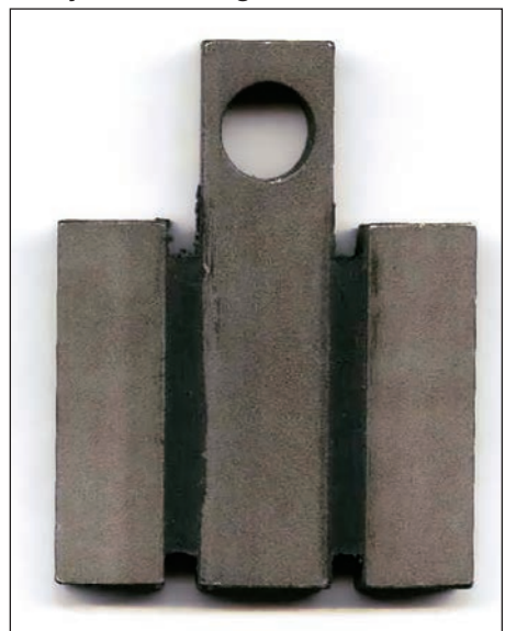
Fig. 3: Double lap shear specimen used for dynamic testing.
