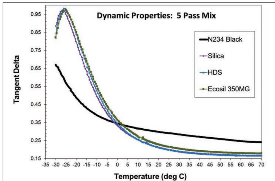
**Fig. 17. Temperature sweeps for N234-control, HDS and Ecosil-filled treads for 3-pass and 5-pass mixes.**
