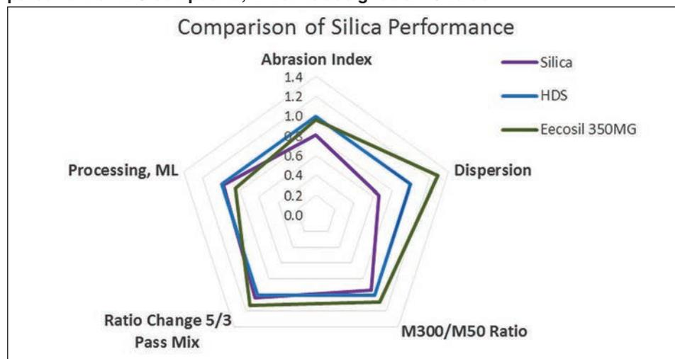
**Fig. 20. Radar graph of important dynamic properties for silica-filled treads compared to the HDS compound, which is assigned a 1.0 value.**
