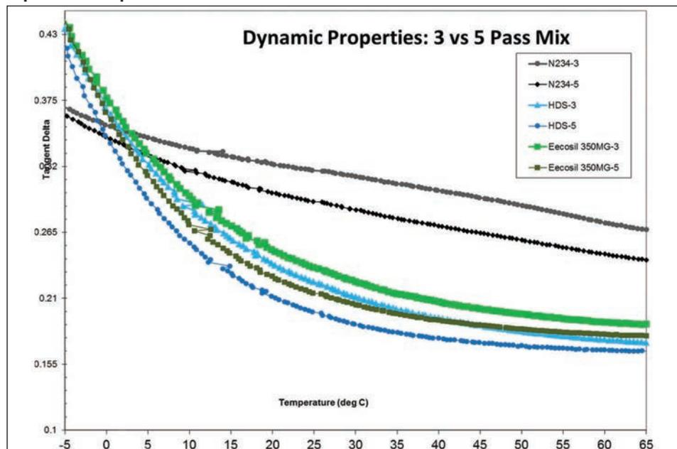
**Fig. 18. Temperature sweeps for N234-control and silica-filled treads.**
