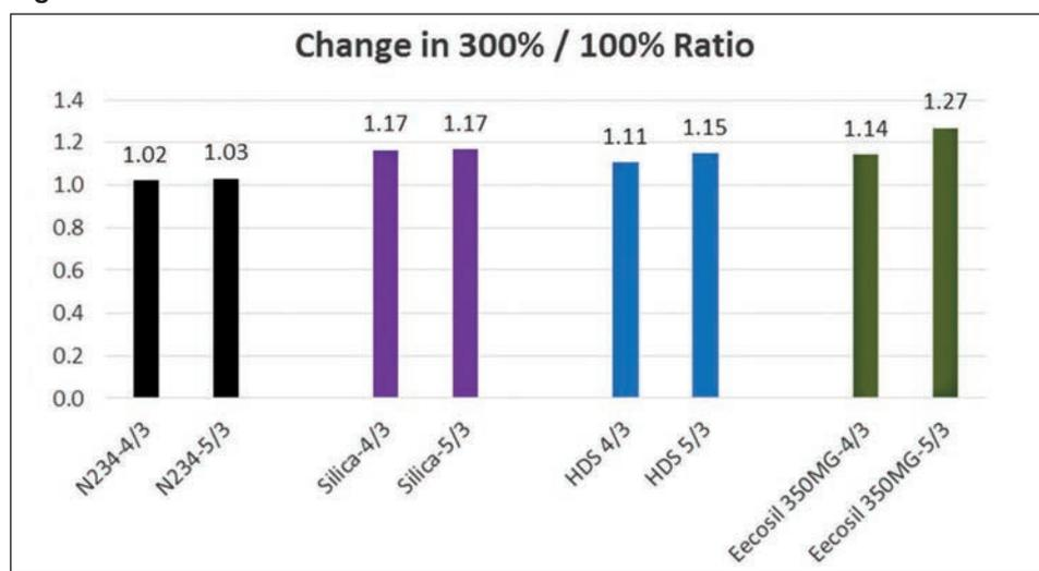
Fig. 9. M300/M50 ratios for N234-control and silica-filled treads.
