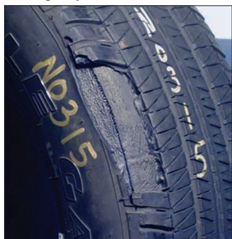
Fig. 13: Photograph of a tire displaying belt edge exposed = BEE.
