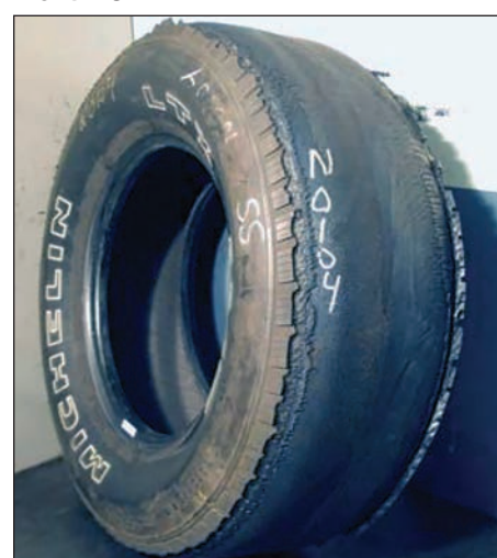
Fig. 18: Photograph of a tire displaying complete tread to belt No. 2 detachment = CT+B2D.
