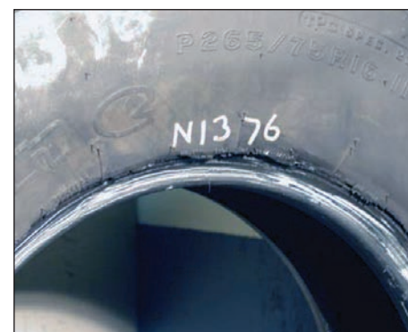
Fig. 3: Photograph of a tire displaying a bead turnout rupture = BdTuR.
