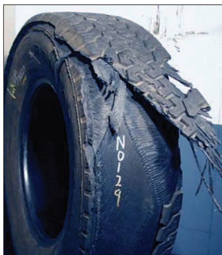
Fig. 18: Photograph of a tire displaying complete tread to belt No. 2 detachment = CT+B2D.
