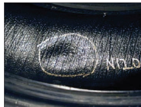
Fig. 5: Photograph of a tire displaying an innerliner split = ILSplit.
