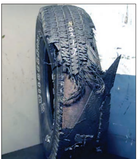
Fig. 16: Photograph displaying belt No. 1 to carcass detachment = B1P1D.
