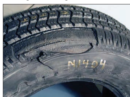
Fig. 14: Photograph of a tire displaying belt edge loosening = BEL.
