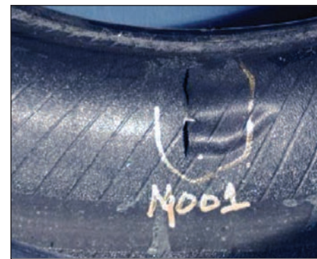
Fig. 5: Photograph of a tire displaying an innerliner split = ILSplit.
