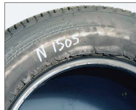
Fig. 3: Photograph of a tire displaying a bead turnout rupture = BdTuR.
