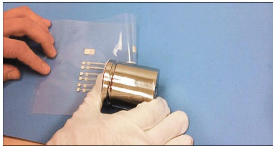
Fig. 7: ISO 7854 crumple test.
